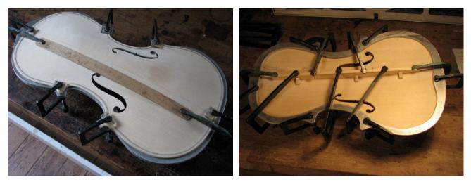
The top image shows my baroque style bass bar clamps. They were made of plywood some thirty years ago and still have enough spring. You can use them for modern bars if you plane an apex on top of the bass bar. I have glued a strip of leather on the side that comes up against the belly arching. The bottom image show the modern clamps used in this article laid out for clamping.
