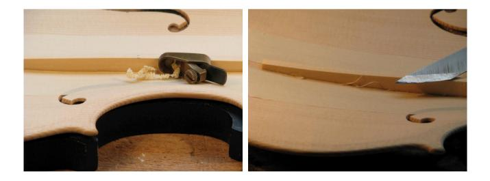
The first picture of the bars end shows the right side of the taper completed. The second shows both sides tapered. This work should be finished as accurately as possible. The better the finish at this stage, the easier it will be to create the bar's final shape.
