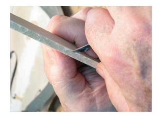
Once the bar fits perfectly (perfect is good for the health of the violin, we don't fit sound posts with 'spring' because this also damages the belly) the bar is lightly clamped in place. The two rules of woodworking are: measure twice and cut once and always clamp dry before you glue.
