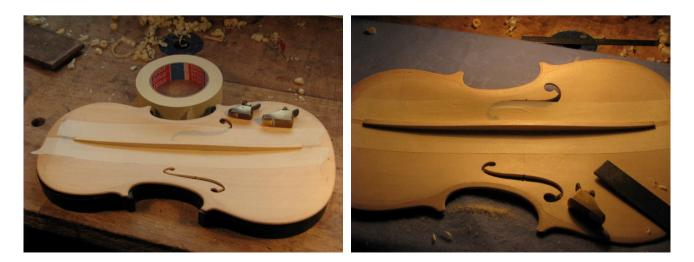
I plane the long side profile roughly to shape making the bridge position the highest point. I finish the upper bout profile slightly more scooped while leaving the lower bout profile a little fuller. I call this the 'fastback' look. Sometimes, using a draw filling action, I finish the top shape with a rasp, especially if I need a tighter curve. However, in spite of the scooped look, at no point does the bar become thinner than it becomes at either end.
