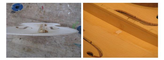
When working on the bar shape it is easy to damage the belly with planes and knives. For this reason, I run two strips of masking tape down either side of the bar. (I understand Andrea Amati invented masking tape in 1567 after he had some trouble with one of the decorated instrument made for Charles IX.)
