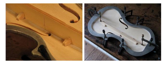
At this stage I clean off the chalk and size the bar and belly before leaving it to dry for at least four hours. Once the glue is dry, I quickly refit the bar with chalk before finally gluing it in position. During the dry run, I always mark on the bar where the clamps are to be placed and lay out the clamps in their correct positions.
